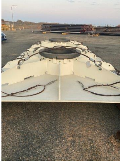
Mud Mats for Conductor Support
